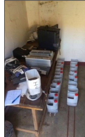
Fig. 16. After two days the samples are weighed (right section: remaining samples standing on rails) 122
