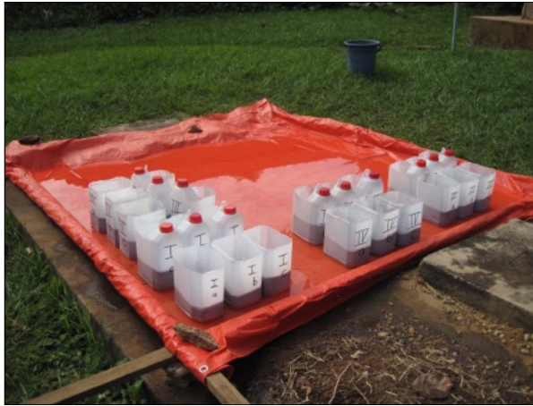
Fig. 15. Soil samples being saturated with water 121
