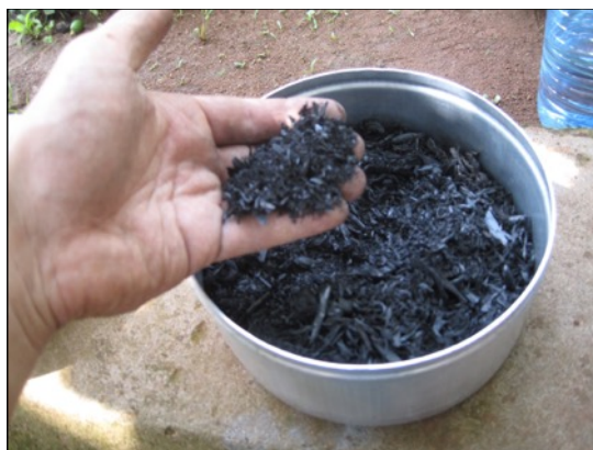
Fig. 14. Yielded WAHY-BC after cooling down. 118
