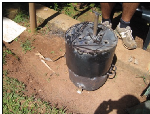
Fig. 13. The mounted lid creates the heating chamber. 117
