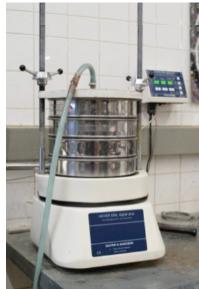
Fig. 8. Sieve tower on a vibration device. 107
