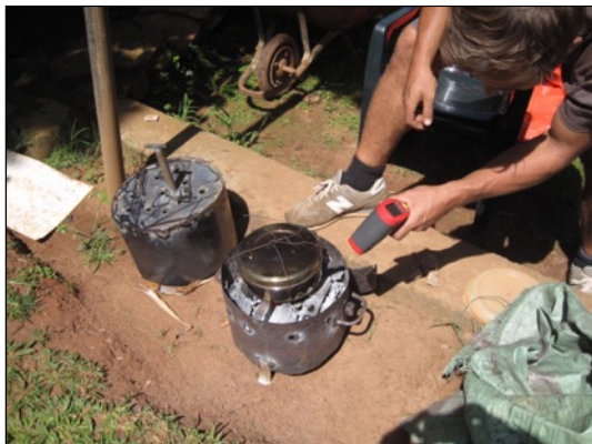
Fig. 12. Cylinder upon the burning chamber, while the temperature in the burning chamber is checked. 116
